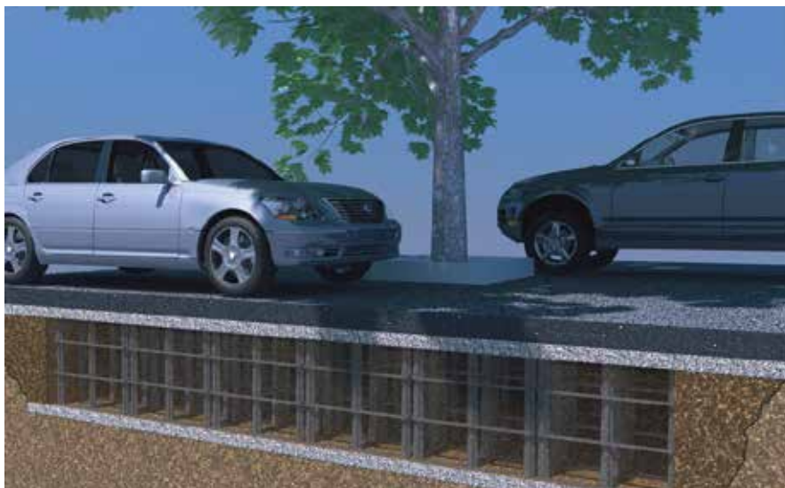
FIGURE 30: Example of a modular support structure underneath a parking lot. Image © deeproot
