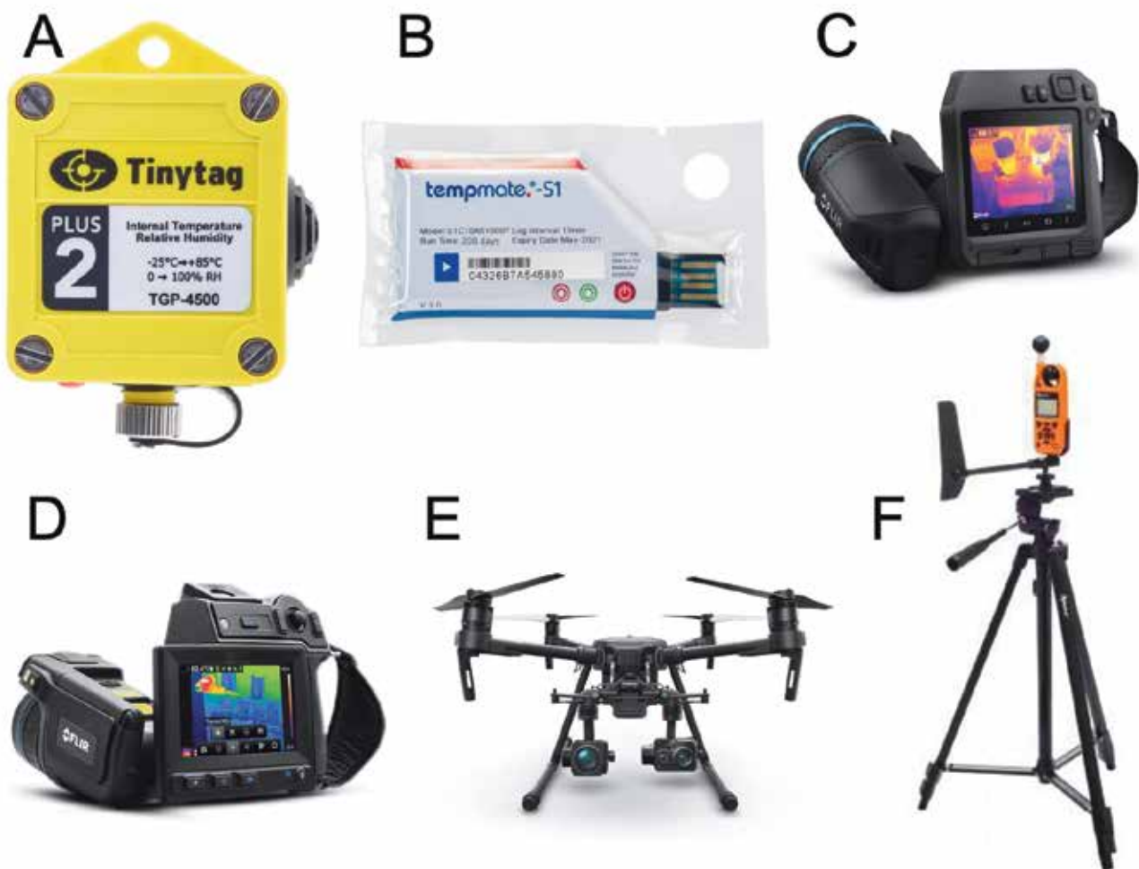
FIGURE 5: Devices used to document air and surface temperatures in the three car park projects. A: TinyTag logger (TGP-4500) for continuous measurements of air temperature; B: Tempmate (S1 V2) logger for continuous measurements of air temperature; FLIR T540 (C), FLIR T840 (D) for ground-based spot measurements of surface temperatures; E: DJI M210 aircraft and FLIR Zenmuse-XT2 camera for periodic aerial measurements of surface temperatures; F: Kestrel 5400 Heat Stress Tracker with black globe thermometer on a tripod.
