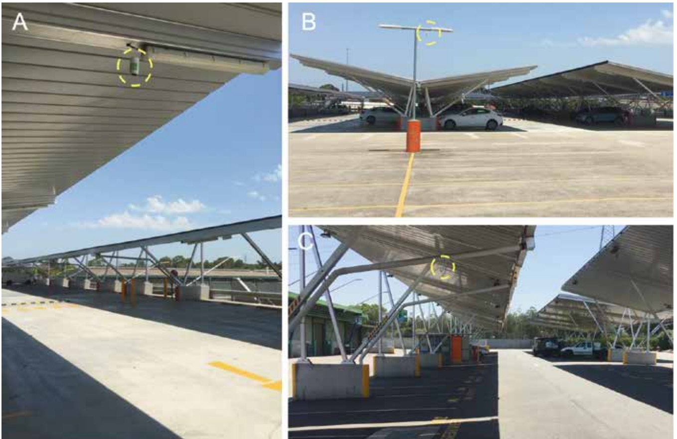
FIGURE 25: Examples of positioning the custom-made loggers underneath the solar panels at locations A and B. Panel A: shade at location B. Panel B: Full sun and location B. Panel C: Shade at location A. Image © S. Pfautsch
