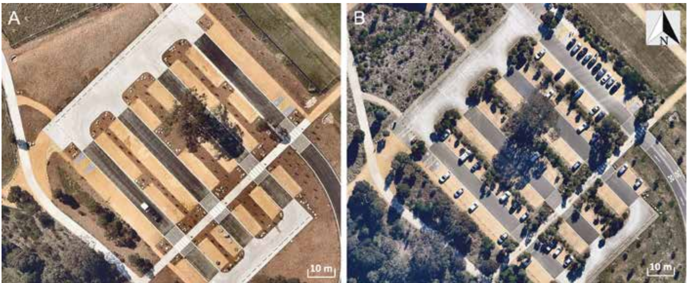
FIGURE 27: A car park made of locally sourced crushed sandstone in Bungarribee Super Park in Western Sydney Parklands, NSW. The two images depict the car park shortly after construction (A: October 2015) and six years later (B: August 2021). Images extracted from Nearmaps.
