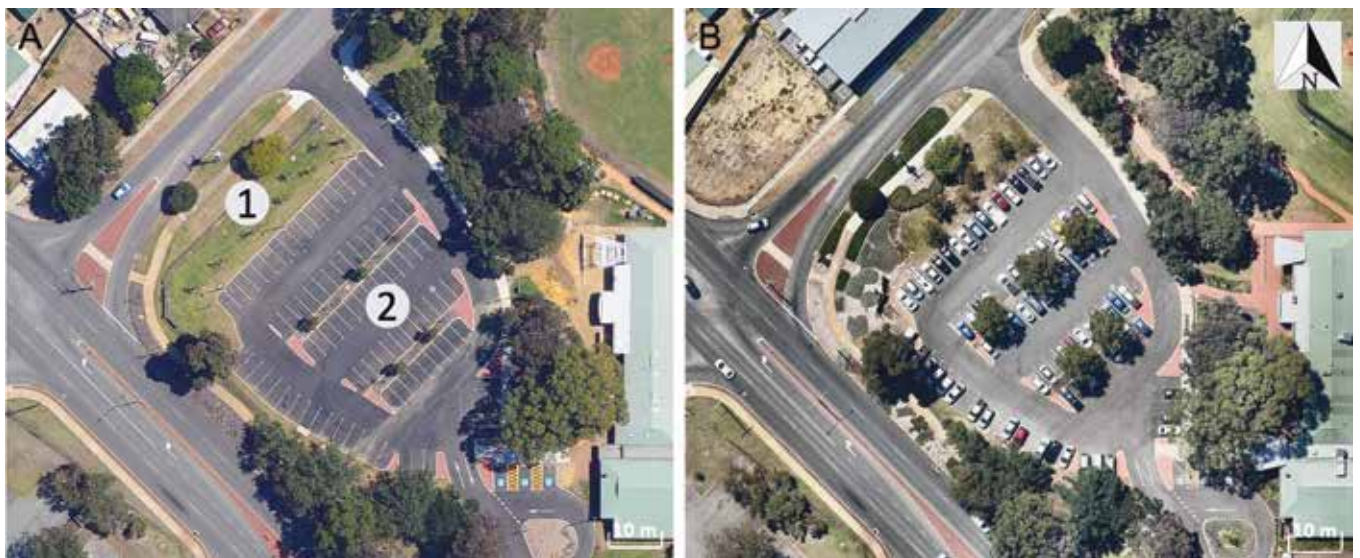
FIGURE 28: A car park in Forster Park in the City of Belmont, Perth, WA. The two images show trees after planting in January 2013 (A) and well-grown tree crowns in February 2019 (B). These images illustrate the effect of the planting method on the size of the canopy. 1: Trees were planted traditionally in the open ground. 2: Trees planted in the soil vault system. Images extracted from Nearmap.
