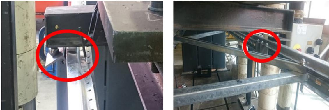
**Figure 4-8: Crippling of load points: (A) Typical crippling at flanges; (B) Specific crippling reinforcement.**
