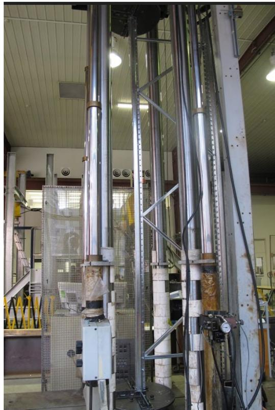
**Figure 3-10: 3600 mm specimen and boundary conditions.**
